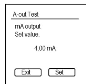
4. Confirm the value with the Measure/Enter button (Set). A signal will be send to the external device, which is translating it into pH.
