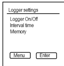
**Remark:** If the sensor is in logging mode, it is not possible to communicate with the sensor through an external device, e.g. a computer. Logging has to be stopped first to communicate with the sensor. Nevertheless, by pressing the Measure/Enter button the last measured value will be visible on the display.
