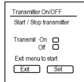
5. Exit menu with the Menu/Exit button. Transmitting will start automatically.
