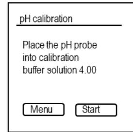
5. Keep the probe in pH 4 buffer until you are instructed to place it into pH 7 buffer.
