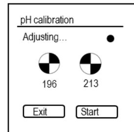
7. Press the Measure/Enter button (Start) and wait until the sensor finishes the calibration.
