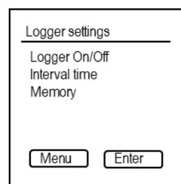
**Remark:** If the sensor is in logging mode, it is not possible to communicate with the sensor through an external device, e.g. a computer. Logging must be stopped first to communicate with the sensor. Nevertheless, by pressing the Measure/Enter button the last measured value will be visible on the display.
