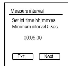
5. Use the Measure/Enter button (Next) to navigate to the next position in time (hh:mm:ss).
