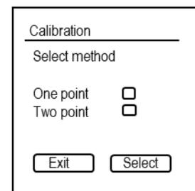
The temperature is always the first parameter to be calibrated. A temperature calibration is advisable for accurate measurements but can be skipped by pressing the Menu/Exit button (Skip), if wanted. If so, the sensor will automatically ask for the next parameter to be calibrated.
