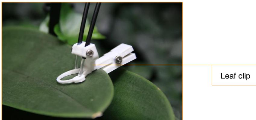
The FluoMini Pro Optical Eff% + PAR Sensor is provided with a leaf clip for the measurements on leaves of living plants.
