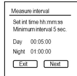
**Remark:** The interval time for the digital FluoMini Pro Eff% + PAR Sensor can be controlled through an external device. In this case, the interval times set within this menu are not valid.
