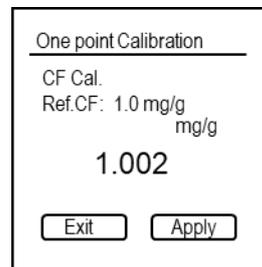
4. Wait until the measured value on the display is stable and press the Measure/Enter button (Apply).
