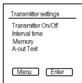
turned on and off, the interval time of the measurements can be set, stored data erased and the analog output being tested. Use the Up and Down buttons to navigate to the desired submenu. To enter a submenu, press the Measure/Enter button.
