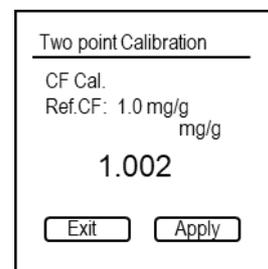
1. Use the Up and Down buttons to set the reference value (noted on the calibration plug).
