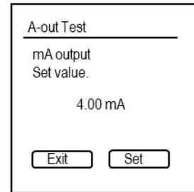
5. Compare this value with the CF on the external device. Here, 4 – 20 mA are translated to 0 – 50000 counts or 0 – 20 mg/g. Therefore, a change of 1 mA relates to a change of 3125 counts or 1.25 mg/g.
